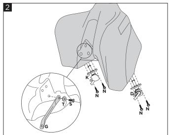
Apply the brackets (G) to the Acerbis tank (A), on both sides, using the screws (S) and washers (T). Fit the petcocks (D) using the screws (N) and place the tank on the bike.
