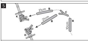
Connect the petcocks (D) to the carburetor using the Y fitting (C) and the pipe rubber (B), cut to the measurements indicated in the figure.
