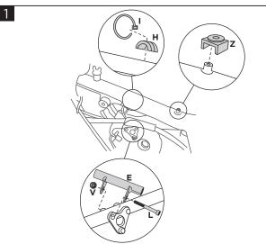
Remove the rubber support (Z) from the original tank and reassemble it on the frame. Apply the rubber support (H) to the frame and fix it with the zip tie (I). Remove the original screw and nut and mount the spacer (E) using the supplied screw (L) and the original nut (V) as shown in the figure.
