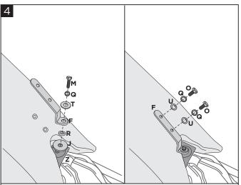
Mount the bracket (F) on the rubber (Z) mounted on the frame, using the bushing (R), the washer (T), the washer (Q) and the screw (M). Fix the bracket to the Acerbis tank using the washers (U), washers (Q) and screws (O).
